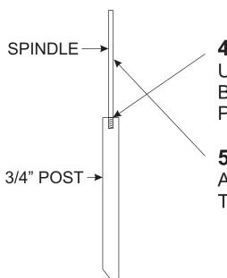
USE LOCTITE ON THREADS OF SMALL SPINDLE BEFORE SCREWING INTO 3/4" ROD. THIS WILL PREVENT IT FROM BACKING OUT.
