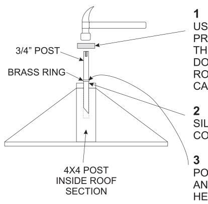
USING A BLOCK OF WOOD TO PREVENT DAMAGE TO THE TOP OF THE POST. GENTLY TAP 3/4" ROD DOWN WITH A HAMMER UNTIL ROD SEATS INTO 4X4 AND YOU CANT TURN POST BY HAND.
